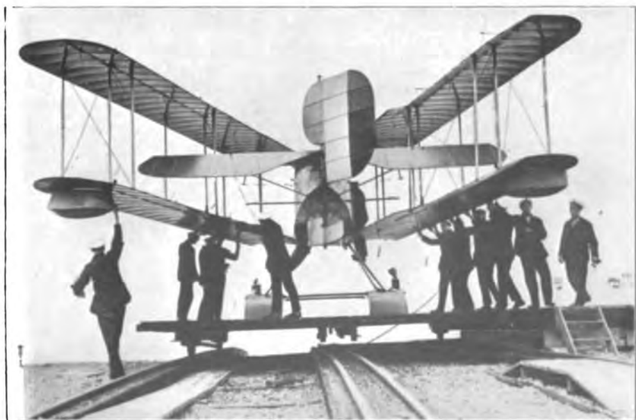
A British Seaplane with Folding Wings
