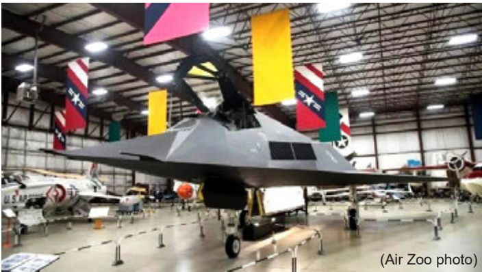
(Above left) The Lockheed F-117 presented a unique restoration challenge in that the still-classified radar absorbing material in the leading edge of the wing and other areas was removed prior to delivery. Some creative engineering was required to design and fabricate alternate replacements. (Right) One of the museum volunteers was the crew chief on this F-104C (56-0898 ) in Vietnam.
