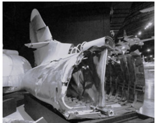
The XF-90 survived the first blast relatively intact. But placement closer to ground zero for the follow-on shots did her in.
