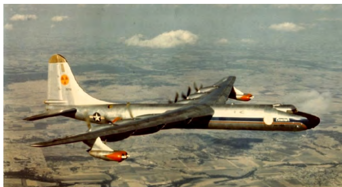
The NB-36H (51-5712) carried a nuclear reactor but retained its conventional piston/jet propulsion system. The cockpit was shielded with lead to protect the crew from radiation. (USAF photo)
