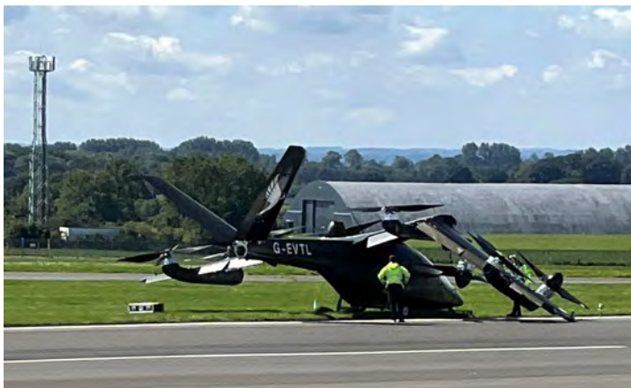
Vertical Aerospace's VX4 was seriously damaged when prop blade separated during a test flight. (Photo: dronedj.com)
