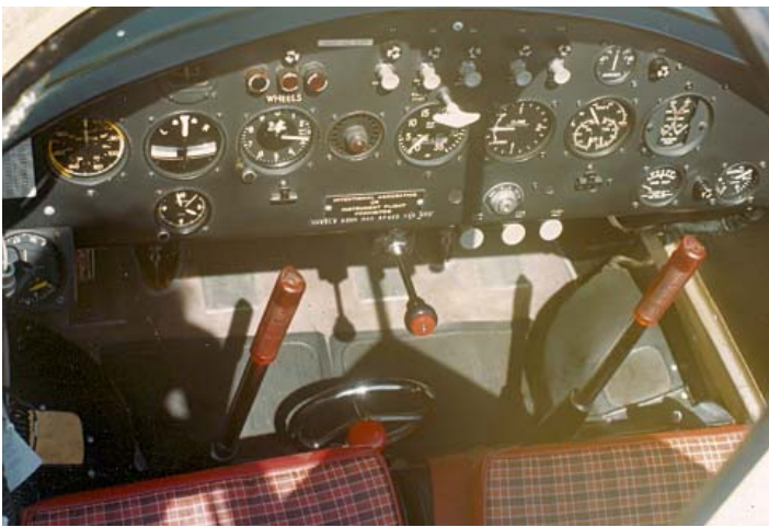
Cockpit of N281W present day. Aircraft has a full electrical system including landing gear aural and visual warnings. The chrome wheel in between seats is for landing gear retraction; the red knob behind it is locking lever.
