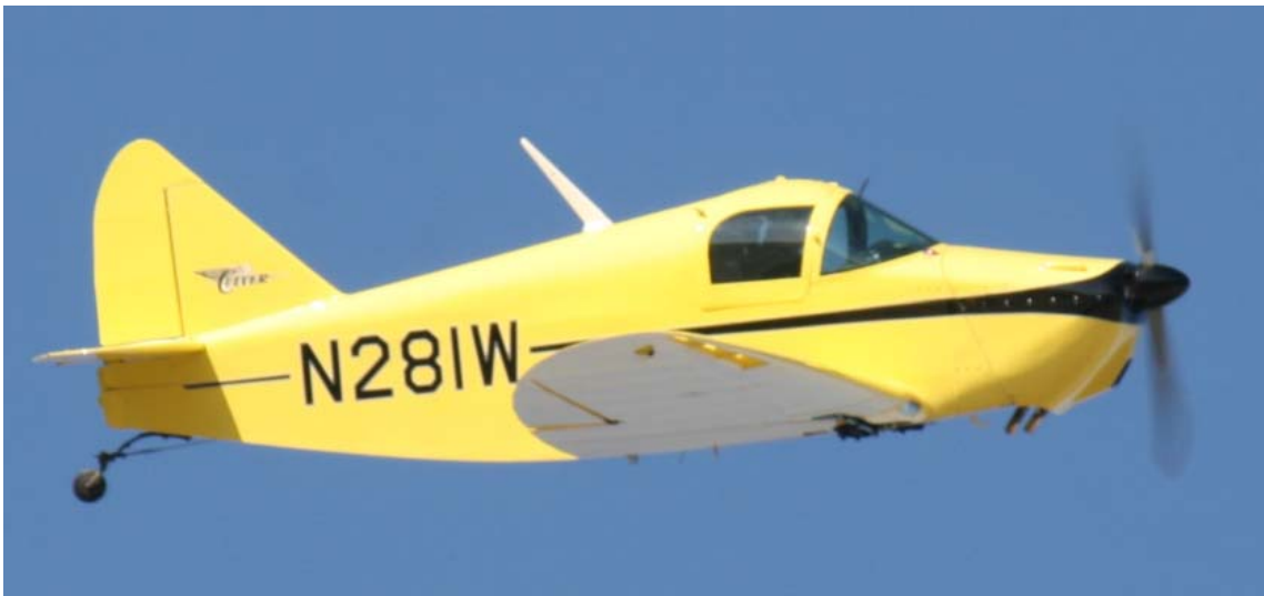
Jim Rezich departs in N281W. The original registration number is reserved by Jim for when the airplane is repainted in the original colors. Note the Freedman-Burnham ground adjustable wooded blade propeller; it has been replaced with a McCauley aluminum propeller.
