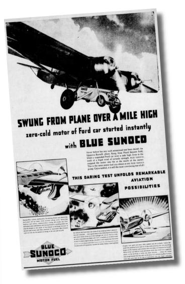
would have been at road speeds on the ground. But I never did get the big bus up to normal speed. The air resistance of the car underneath held it down to a hundred and thirty. The effect on the controls was three degrees. To counteract the tendency of the tail to rise and the nose to swing down, I had to keep the stabilizer depressed three degrees below normal."
