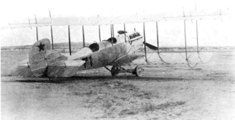
Curtiss R-2, with VX engine of 160 hp, and red star on rudder, device used in 1915-16 by Signal Corps. (Photo—Curtiss, courtesy Peter M. Bowers).
