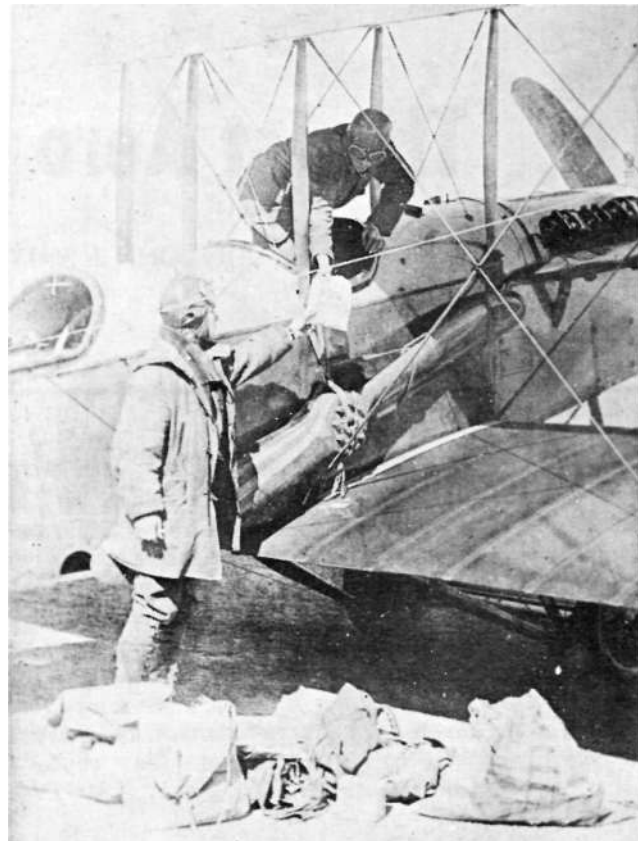
Mail and dispatches were carried on many trips in Mexico, and the prevalence of the propeller problem is shown here. A Curtiss R-2 is loaded, and the spare prop lashed to the sides of the fuselage. At one time a special shop was set up for a factory-trained crew to provide propellers at Columbus, N.M. (Photo—Joseph Gastreich album, courtesy of John R. Wells).
