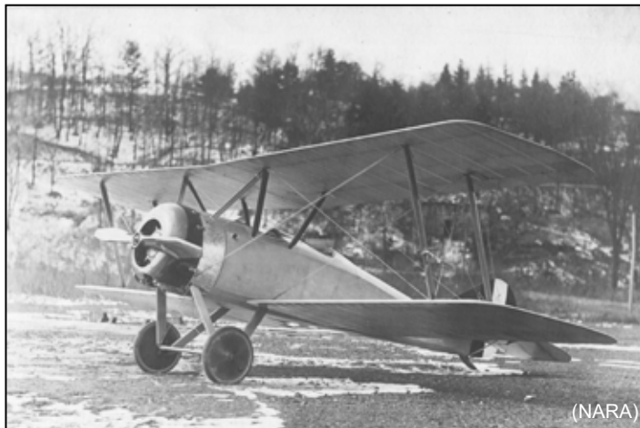
The S-6 was a two-seat derivative of the Tommy. The striped rudder was probably surplus from wartime S-4 production.
