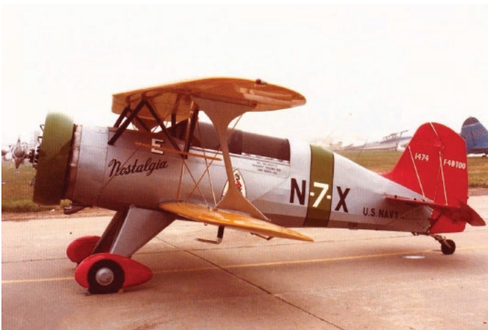
Highly unusual (Continental R-670 engine) Stolp Starduster Too (N7X) owned by Wil Neubert, mimicking a 1930s Boeing F4B. Photographed at Watsonville, Calif., May 24, 1975
