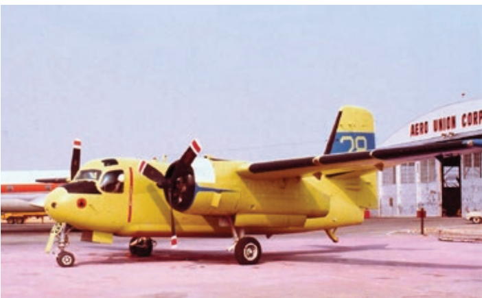
Unidentified Grumman S2F converted to a fire bomber. Seen at Chico, Calif., Oct. 24, 1974.
